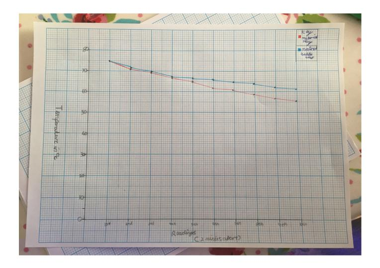
I tried two different types of materials for my little dormouse. One was a natural material (hay) and the other (bubble wrap\*) was a man-made material. The graph (above) shows that the bubble wrap kept my little dormouse the cosiest for the longest.
